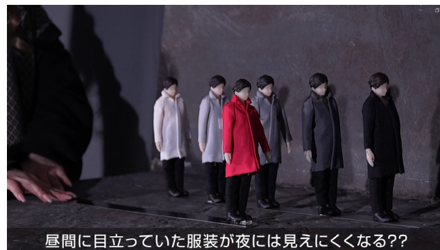
昼間に目立っていた服装が夜には見えにくくなる?? Visibility evaluation experiment of chromatic colors of pedestrian clothing using character figures and an actual car
