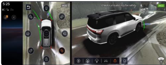
Intelligent Around view monitor (25MY QX80~) 3D View and Invisible hood view.
