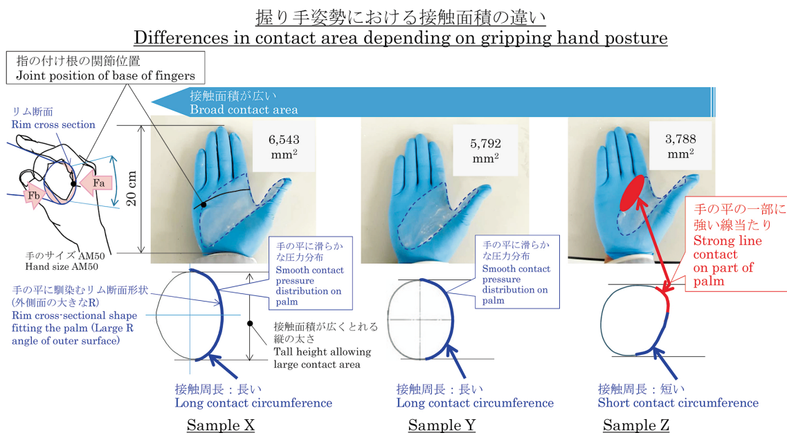
図-5 握り手の接触面積の比較 Fig. 5 Comparison of contact area of gripping hand
