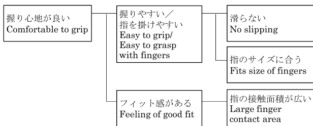
図-2 握り心地の良い形状の構成要因 Fig. 2 Factors in ease of gripping
