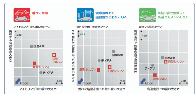
図-6 走行シーンによる静粛性比較 Fig. 6 Quietness by driving scene
