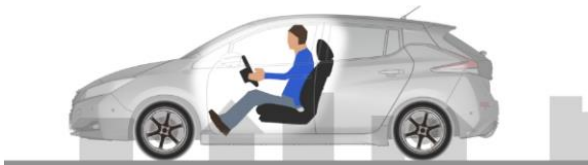
Fig.6 Attitude control when decelerated
