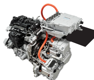
Fig.2 Appearance of e-POWER
