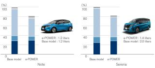
Production & logistics Fuel & electricity production Usage Maintenance ELV Production in Japan, 100,000 km driven in Japan (basis for comparison).
