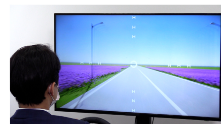
Effective field of view measurement system developed by the Traffic Safety Future Creation Lab
