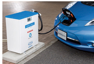
"LEAF to Home" with EV power station developed by Nichicon Corp.
