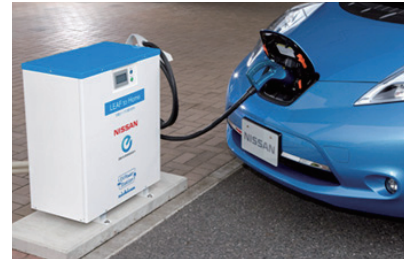
The “LEAF to Home” system in action, using the EV Power Station released by Nichikon in June 2012
