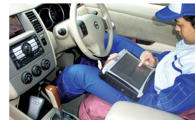
Nissan's Consult system helps service personnel identify problems in complex modern cars.
