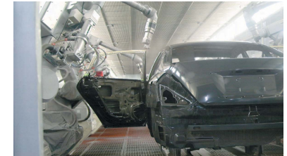
A Kyushu Plant line switched to water-based paint, producing less VOCs.
