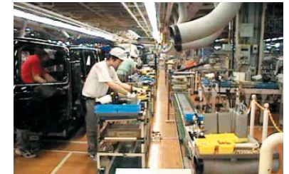
Before the "strike zone" approach was adopted, workers walked to a shelf for parts and back to the vehicle (above); now the needed parts are within easy reach (below).
