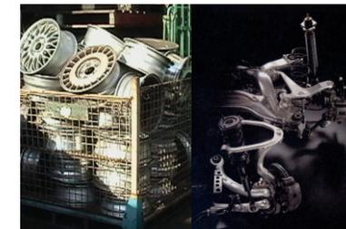
Suspension parts recycled from aluminum wheels
