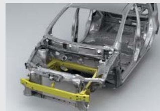
A crash-compatible Zone Body construction (Note)
