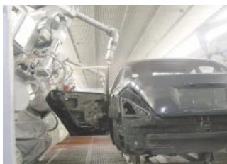
A line switched to water-based paint, producing less VOCs at Kyushu Plant
