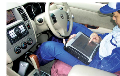
Nissan's Consult system helps service personnel identify problems in complex modern cars.
