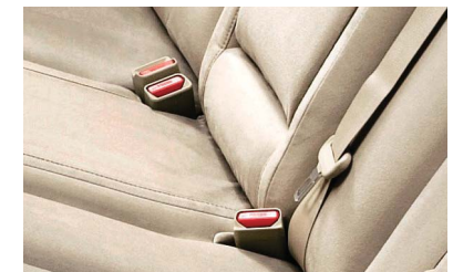
Self-standing buckles make seatbelt use easier for passengers in the rear seats.
