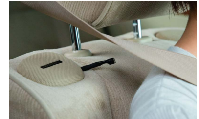
An alcohol odor detection device in the driver's seat aims to reduce driving under the influence.
