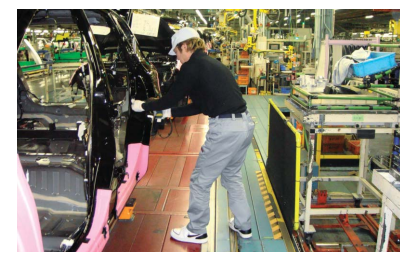
Workers had to squat to assemble parts before introduction of the "strike zone" approach (above); these stressful positions are no longer needed thanks to conveyors that can raise and lower the cars being worked on (below).
