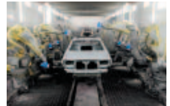
Water-based paint line
